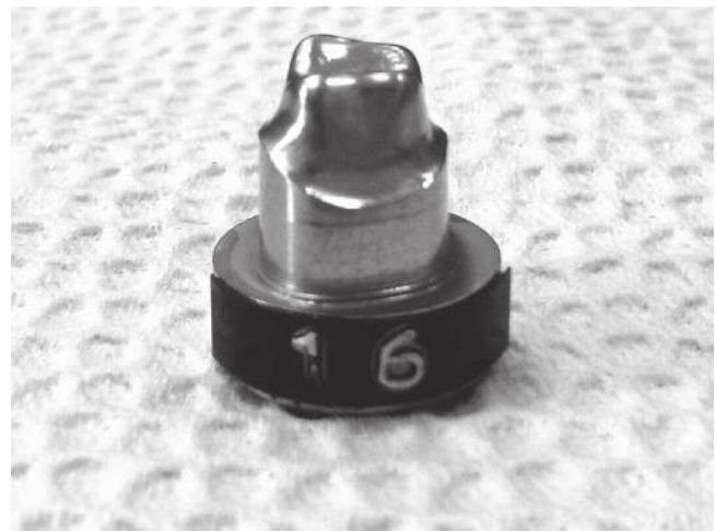
Fig. 1. Titanium master model (1.2 mm and 360° chamfer form preparation was made on a maxillary right first molar).
