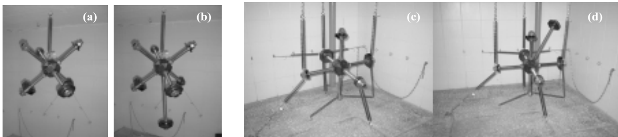
Fig. 3. Suspension set-ups used for the application of: IRM (a),(b) and MM and DPPIM methods (c),(d).
