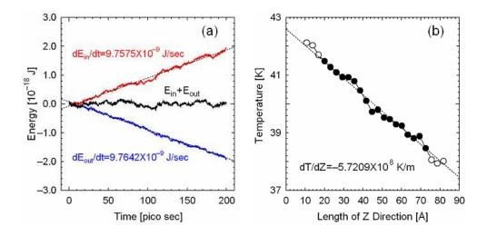
Fig. 5. (a) Heat flux and (b) temperature profile obtained by using the velocity scaling method at  $T_{ave} = 40 \text{ K}$  for a system size of 68 Å x 59 Å x 55 Å.
