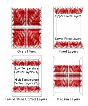
FIG. 2. The simulation system with an adiabatic wall. The size of a system is the example of 18 x 18 molecules in the x-y plane and 30 layers in the z direction. The heat energy flows up (+z direction).
