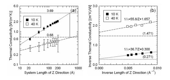
Fig. 6. Dependences of the thermal conductivities on the system size : (a) log-log scale and (b) inverse scale.
