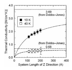
FIG. 7. Variation of the thermal conductivity of solid argon films with the thickness.
