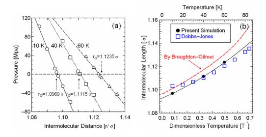
Fig. 4. (a) Pressure as a function of the intermolecular length and (b) intermolecular length as a function of the dimensionless temperature for a free-standing state.
