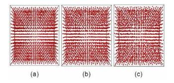
FIG. 3. Simulation system for calculating the system pressure: (a) 10 K, (b) 40 K, and (c) 60 K. The size of the system is 12 x 12 x 18, the boundary conditions of which are 3-dimensional periodic boundary conditions.
