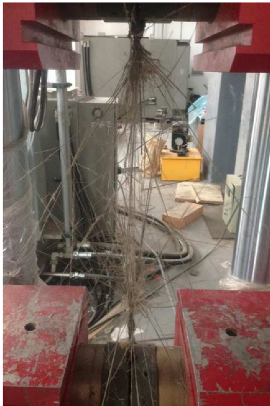
Figure 26: Failure mode in the short-term tensile test [103].
