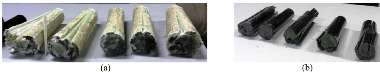
Figure 8: Observed failure modes in tested FRP bars: (a) GFRP and (b) CFRP [53].
