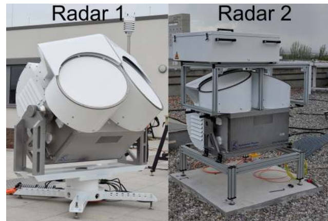
Figure 1. Impressions of the two frequency-modulated continuous wave (FMCW) W-band radars used in this study, as indicated in Table 2. Images courtesy of the radar owners.
