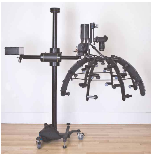
Figure 2 The Worcester Art Museum's portable fixed-light array RTI dome (photo by Marlin Lum, Cultural Heritage Imaging).
