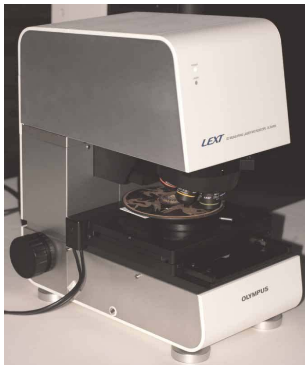
Figure 4 LEXT OLS4000 3D measuring laser microscope manufactured by Olympus. Pictured on the instrument stage is the lid from the Pyxis by the Eretria Painter, c. 430 BCE (WAM 1935.148), which was part of this research.
