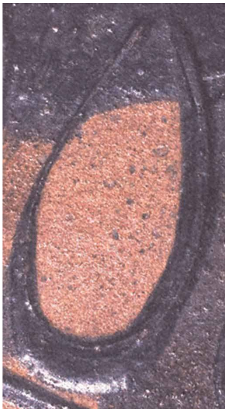
Figure 10 Confocal image of a looped line in the headdress of Thetis. The field of view is about 4.0 \times 2.2 mm and the image was stitched from eight individual area scans taken with a 5x objective.
