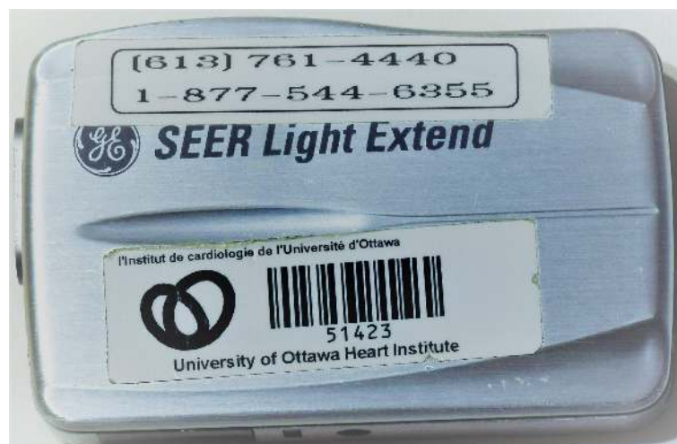
Figure 3.4: The General Electric Seer Light Extend Holter monitor was the source of the ECG Signal.
