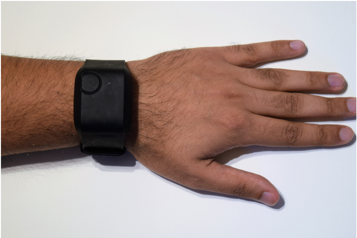
Figure 3.1: The Empatica E4 wristband was the source of the PPG Signal.
