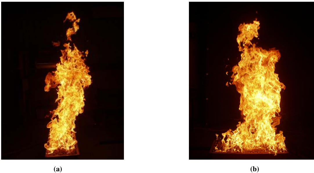
Figure 28: Typical view of a 300 kW fire from the 3:1 aspect ratio burner when viewed from (a) the side and (b) the front
