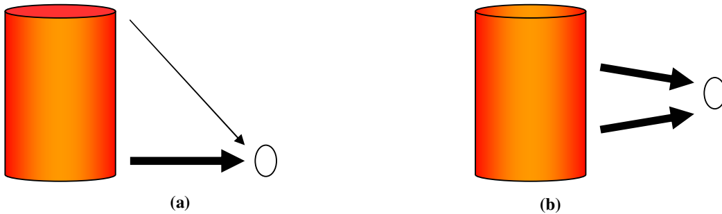
Figure 31: Schematic of radiation from a cylindrical fire to a target located at (a) the base height of the flame and (b) the mid-height of the flame. The thickness of the arrows represent the amount of radiation being received from different areas of the fire (not to scale)
