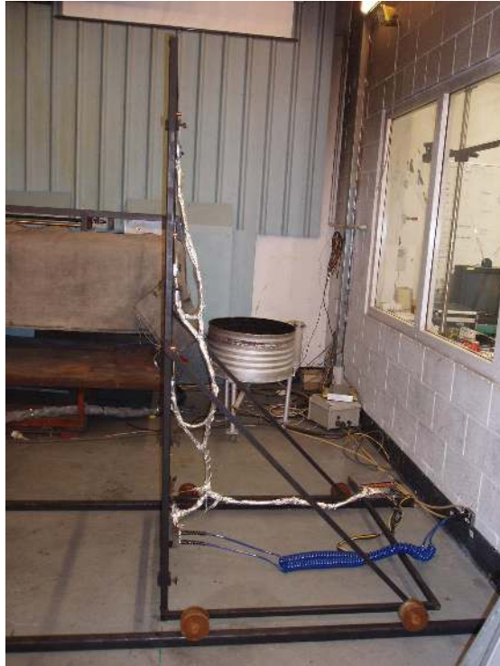
Figure 15: Side view of heat flux gauge trolley on its tracks
