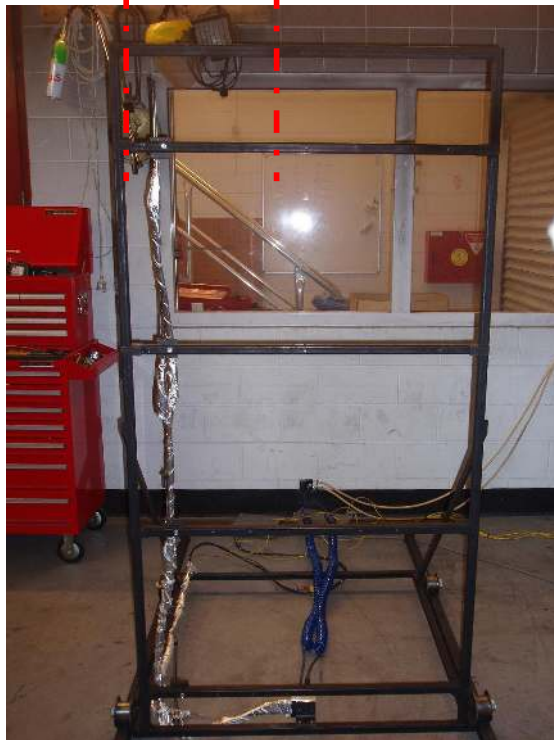
Figure 16: Front view of heat flux gauge trolley with offset and central gauge positions indicated
