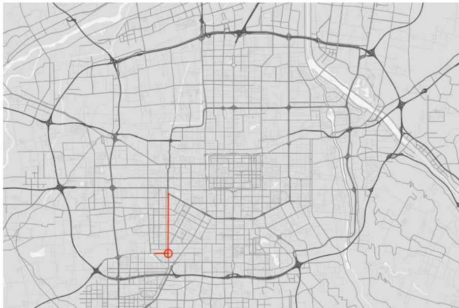
Figure 2. The investigated intersection location scheme. The investigated intersection is a T-intersection and located in the center of Xi'an CBD district. The arterial street is a North–South seven-lane road, and the collector street is a West–East seven-lane road.
