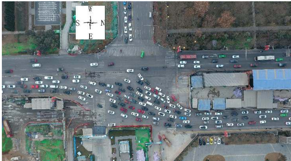
Figure 3. The present situation of the T-intersection. This graphic was taken by a drone at a height of 130 m. A construction site occupies the North part of the intersection and forces operating vehicles to be offset by 28 m. Another construction site occupies half of the road area of the southern road of the intersection. Coordinates: 108.889684, 34.205037.
