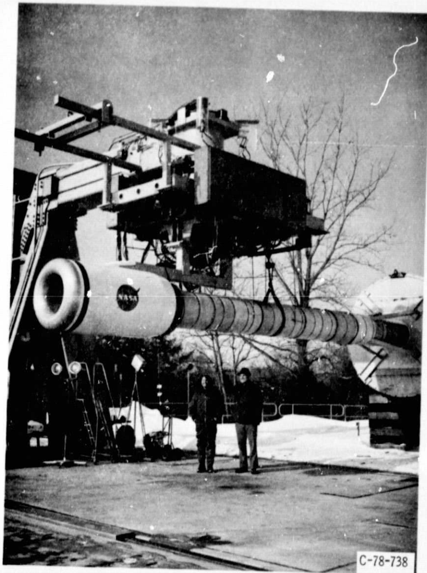
Figure 3. - JT15D engine mounted on test stand.
