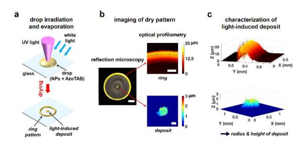
Figure 1. Light-generated particle deposits from evaporating sessile drops of colloidal suspensions. a) Schematic of the experiment. A 7  $\mu$ L sessile drop containing AzoTAB cationic photosensitive surfactants (concentration  $C_s$ ) and cationic polystyrene nanoparticles (NPs, 200 nm diameter,
