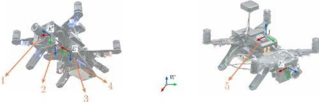
Fig. 3. Representation of coordinate frames on the hardware platform used. (1) Front facing DAVIS 240C, (2) down facing sonar on PX4Flow, (3) down facing DAVIS 240B, (4) NVIDIA TX2 CPU+GPU, (5) Intel® Aero Compute board.
