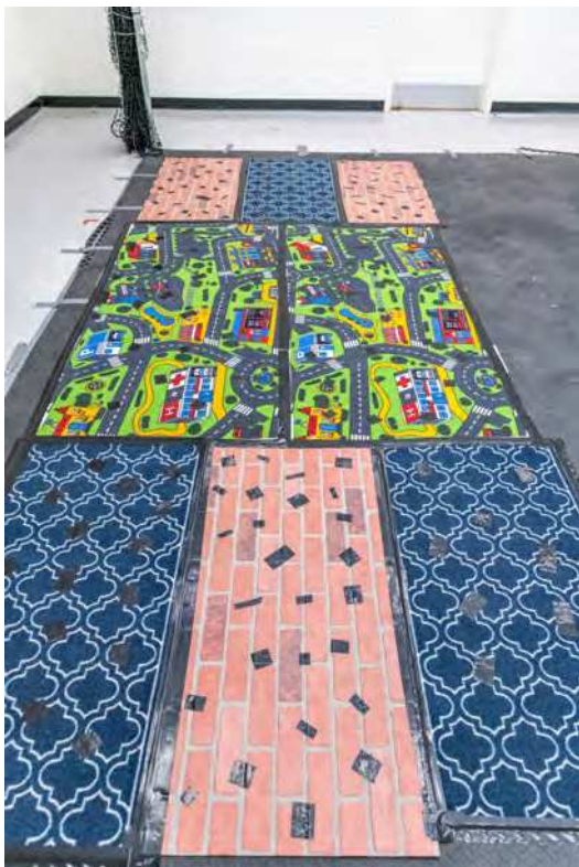
Figure S6. Different textured carpets laid on the ground during real experiments to aid robust homography estimation from EVHomographyNet.
