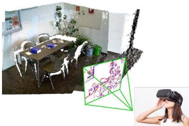
Fig. 1: Sample application: 6-DOF tracking in AR/VR (Augmented or Virtual Reality) scenarios. The pose of the event camera (rigidly attached to a hand or head tracker) is tracked from a previously built photometric depth map (RGB-D) of the scene. Positive and negative events are represented in blue and red, respectively, on the image plane of the event camera.
