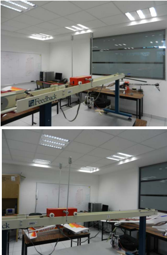
Fig. 2. Inverted pendulum system used for the experiments
