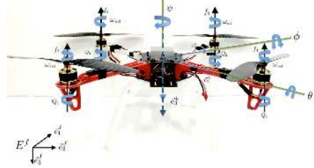
Fig. 4. Quadrotor: fixed frame \mathbf{E}^f = [\vec{e}_1^f, \vec{e}_2^f, \vec{e}_3^f] and body-fixed frame \mathbf{E}^b = [\vec{e}_1^b, \vec{e}_2^b, \vec{e}_3^b]
