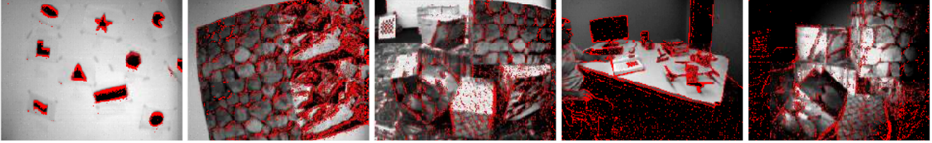
Figure 3: Example images with overlaid events from each sequence. From left to right: shapes, poster, boxes, dynamic, HDR.
