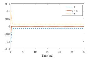
Fig. 8: The tracking error  $y - y_d$
