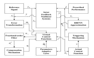
Fig. 1: The flow diagram of FODSC-based fixed-time controller.
