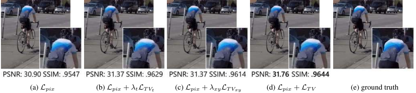
Figure 4: Comparison of different loss functions (simulated single-frame interpolation). \mathcal{L}_{TV} = \lambda_t \mathcal{L}_{TV_t} + \lambda_{xy} \mathcal{L}_{TV_{xy}} .
