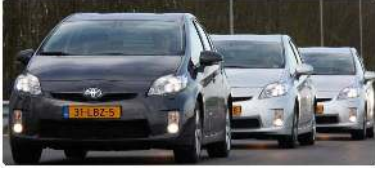
Fig. 6. Benchmark platoon consisting of three passenger cars equipped with long-range radar and DSRC.
