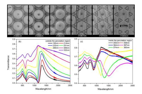
FIG. 1. (a) SEM micrographs of selected CPPS patterns transforming from metallic hole to island arrays. Plots of the measured transmittance vs radiation wavelength for arrays below the percolation threshold (b) and in the percolation region (c).
