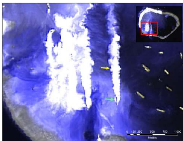
Figure 3. Trailing Hopper Dredges identified by along-side plumes by OLI using bands 8-8-2 in RGB on May 6, 2015. The green and yellow arrows point to a sample dredge and resulting plume, respectively. Landsat-8 imagery courtesy of the U.S. Geological Survey. This image was generated using ERDAS Imagine 2016®, which is a software product owned by Intergraph Corporation doing business as Hexagon Geopatial. © 2016 Hexagon and/or its subsidiaries and affiliates. All rights reserved.
