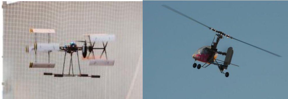
Fig. 8: Left-hand-side, a cyclocopter UAV prototype developed at Northwestern Polytechnical University en China, and right-hand-side, a UAV model of autogyro developed by FUVEX.
