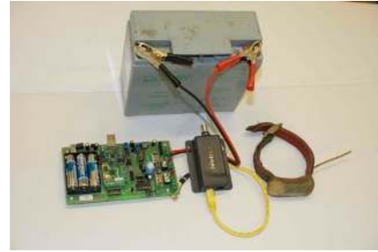
Figure 2. The badger detection node (left) and the active RFID tag, potted in epoxy and mounted on a collar (right).
