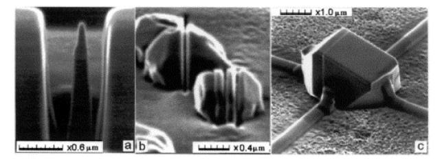
**Figure 14.** Structure fabricated using FIB; (a) nanotip in 1-mm thick ta-C film, (b) nanoscale trenches in diamond microcrystallites, and (c) tungsten contacts. Reprinted with permission from [143]. Copyright 2001, Elsevier.
