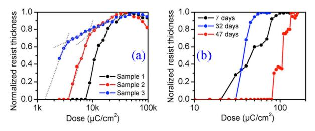
**Figure 16.** (a) EBL contrast curve of different samples at different development time. (b) FHIB contrast curve. Reprinted with permission from [153], Copyright 2018, Elsevier.
