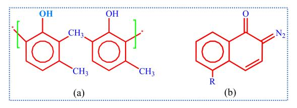
**Figure 3.** Chemical structure of (**a**) novolac polymer; and (**b**) diazoquinones photoactive compound used in most commercial i-line resist.
