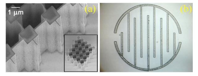
**Figure 15.** (a) Microscope of  $2 \times 2 \mu m^2$  pillars fabricated in SU8 negative resist using p-beam writing with energy of 1 MeV. Reprinted with permission from [146]. Copyright 2003 AIP Publishing. (b) Fabrication of micro walls in PDMS. Reprinted with permission from [147].
