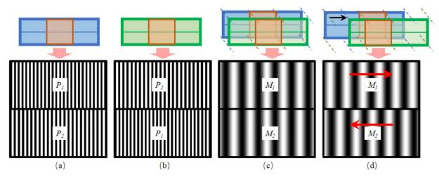
**Figure 13.** (a) Alignment of wafer marks, (b) alignment marks of mask, (c) Fringes of Moire in perfectly aligned wafer and mask and (d) Fringes of Moire in imperfectly aligned mask and wafer. Reprinted with permission from [136]. Copyright 2021, Elsevier.
