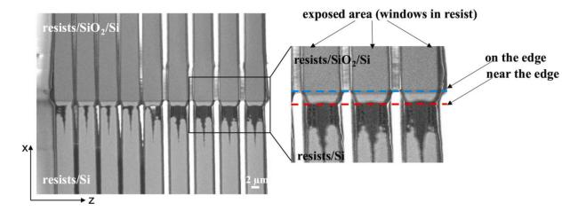
electronics is still a challenge [35], as shown in Figure 4. On the edge and near the edge, the resist gets distorted due to exposure and other factors.
