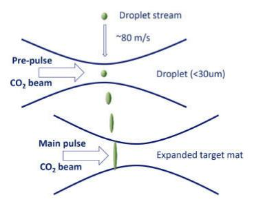
Figure 7. View of EUV generation and target formation. Reprinted with permission from [41].
