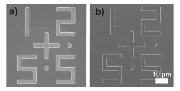
**Figure 10.** Alignment marks in OIR. SEM images at 5 keV showing Al alignment marks on silicon substrates, (**a**) before and (**b**) after condensing 80-nm-thin nonane ice film. Reprinted with permission from [96]. Copyright 2018, Elsevier.
