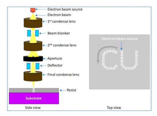
Figure 9. Schematic diagram of EBL system.
