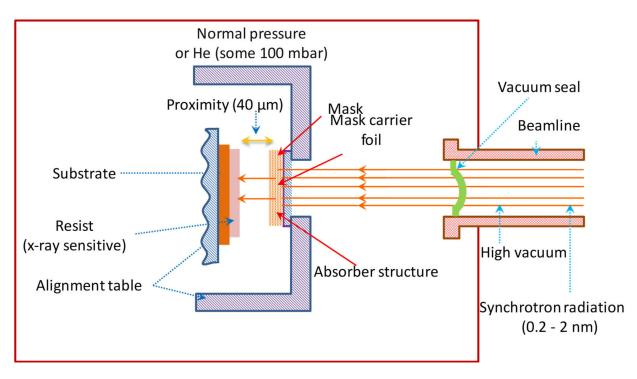
Figure 12. Schematic view of the X-ray lithography system.
