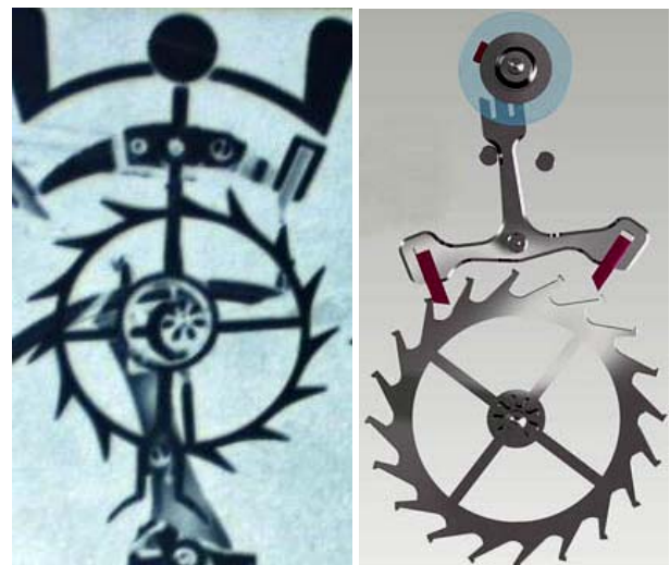
Figure 8. English and Swiss free anchor escapement
