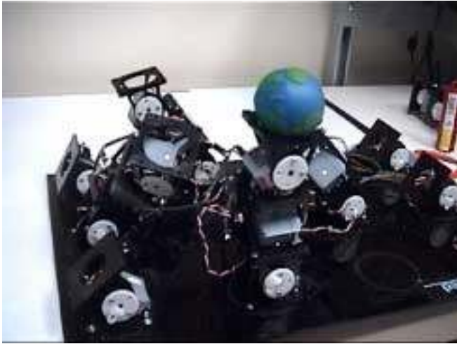
Figure 8: Four arms with three G1 modules each. A small ball is balanced on the end of one arm and passed to the top of an adjacent arm.
