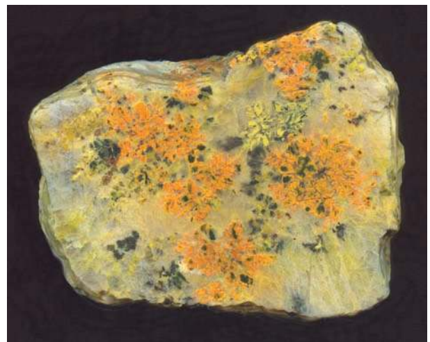
FIGURE 9. Dendritic uraninite mostly altered to “gummite,” which is a mixture of several uranyl minerals, including soddyite, curite, kasolite, uranophane, boltwoodite, and clarkeite (Fron del 1956; Foord et al. 1997). This pegmatitic specimen is from the Ruggles Mine, New Hampshire. Photo courtesy of Robert Lauf. Specimen is 5 cm wide.
