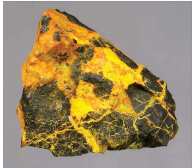
FIGURE 8. Lemon yellow schoepite [(\text{UO}_2)_8\text{O}_2(\text{OH})_{12}\cdot 12\text{H}_2\text{O}] , amber becquerelite [\text{Ca}(\text{UO}_2)_6\text{O}_4(\text{OH})_6\cdot 8\text{H}_2\text{O}] , and orange curite \{\text{Pb}_{3+x}[(\text{UO}_2)_4\text{O}_{4+x}(\text{OH})_{3-x}]_2\cdot 2\text{H}_2\text{O}\} represent progressive alteration of black uraninite ( \text{UO}_2 ) under oxidizing conditions (specimen from Shinkolobwe, Congo). Photo courtesy of Robert Lauf. Specimen is 2 cm in its longest dimension.
