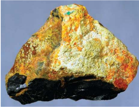
FIGURE 7. Auto-oxidation leads to the formation of Pb-uranyl secondary minerals. Here reddish orange fourmarierite [ \text{Pb}_{1-x}\text{O}_{3-2x}(\text{UO}_2)_4(\text{OH})_{4+2x} \cdot 4\text{H}_2\text{O} ] and bright orange vandendriesscheite [ \text{Pb}_{1.6}(\text{UO}_2)_{10}\text{O}_6(\text{OH})_{11} \cdot 11\text{H}_2\text{O} ], along with pale yellow rutherfordine [ (\text{UO}_2)(\text{CO}_3) ], form a crust of secondary minerals on massive primary uraninite ( \text{UO}_2 ) from Shinkolobwe, Congo. Photo courtesy of Robert Lauf. Specimen is 5 cm wide.
