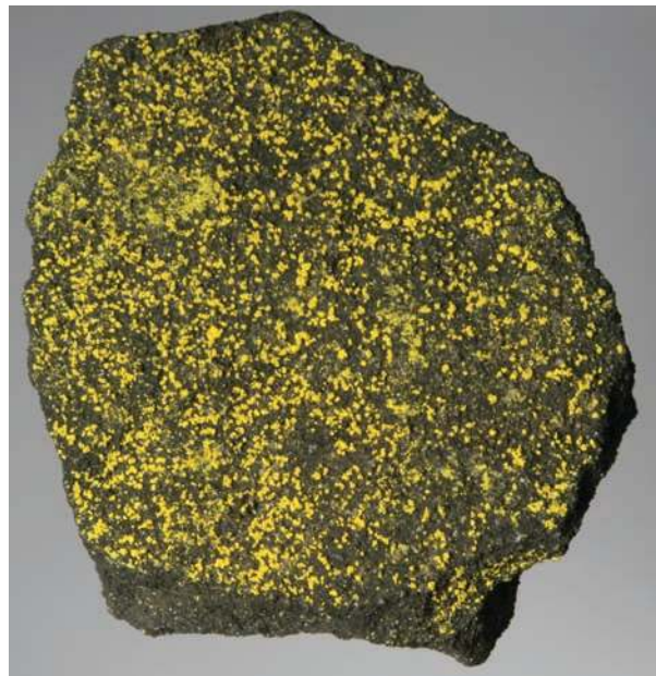
FIGURE 16. Massive black coffinite (ideally USiO_4 ), with a yellow coating of the secondary uranyl sulfate zippelite [ K_3(UO_2)_4(SO_4)_2O_3(OH) \cdot 3H_2O ], formed in the sediment-hosted Grants mineral belt, Section 35 Mine, Jurassic Morrison Formation, New Mexico. Photo courtesy of Robert Lauf. Specimen is 7 cm wide; individual masses of zippelite are up to ~1 mm.
