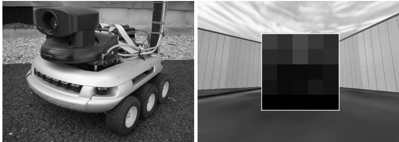
Fig. 1. Left: The original six-wheeled robot Koala equipped with a pan/tilt camera. Right: The robot's perspective in a simulated environment. The robot can access the world with 5 by 5 retina at the center of the image.
