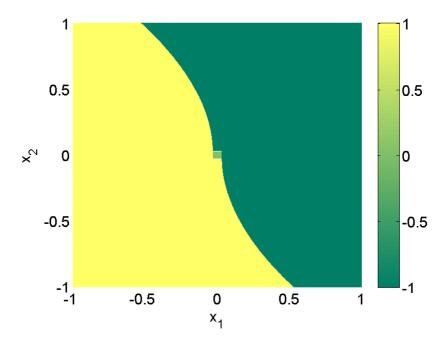
**Figure 5-3:** The optimal control surface for a minimum-time frictionless mass control problem, in which  $x_1 = z$  and  $x_2 = \dot{z}$ . This plot is similar to Figure 5-2(b), but here the value of the control action is presented as a colour. Dark green stands for a control action of -1 and bright yellow represents a control action of +1 (see colour scale).
