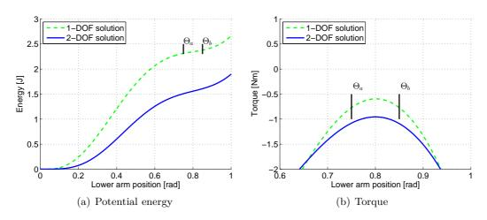
**Figure 5-13:** The potential energy and torque curves corresponding to the best solutions found for the 1-DOF system and the 2-DOF system.
