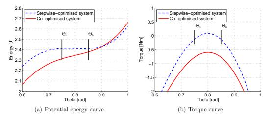
**Figure 5-10:** The potential energy and torque curves of the spring mechanism with parameter values obtained from a stepwise optimisation and an evolutionary optimisation. The EA seems to prefer a bigger torque at the pick-and-place intervals than the minimised torque found in the stepwise optimisation.
