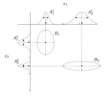
**Figure 4-5:** The free fuzzy controller has membership functions which positions are part of the optimisation problem. Each rule consequent is defined by its own membership functions on the inputs.
