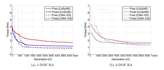
**Figure 5-15:** The average torques of the best solutions found during the optimisation runs of the four controller-algorithm combinations. For both the 1-DOF and 2-DOF RA each combination was tested 20 times. The blue lines represent the optimisation of the fixed fuzzy controller and the red lines that of the free fuzzy controller. One can see that on average the fixed fuzzy controller shows a faster initial converges than the free fuzzy controller.
