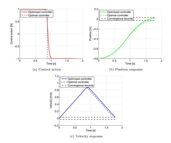
**Figure 5-6:** The control output and state response from the initial state starting at a position of -0.8 m and a velocity of 0 m/s when simulating with the best control solution found during the experiment. The dashed lines represent the optimal control output and corresponding state response, which are very similar to the simulated output.
