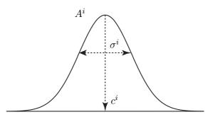
**Figure 4-3:** Gaussian function of the fuzzy term  $A^i$  on the *i*th input defined by its center  $c^i$  and its width  $\sigma^i$ .
