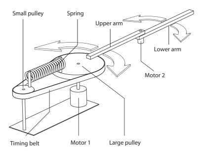
**Figure 3-1:** A drawing of the controlled mechanical system, called the Resonating Arm, which will be optimised in this research. An important part of the Resonating Arm is its spring mechanism, which is represented by the two pulleys, the spring and a timing belt connecting them. Furthermore the systems consists of an upper and lower arm plus two actuators to control both degrees of freedom. (source: [26])
