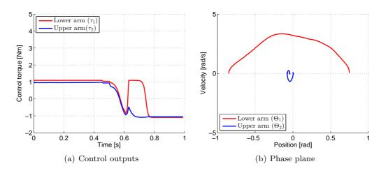
**Figure 5-12:** The control outputs and the phase trajectories of the the actuators and arm angles, respectively, from an initial state of  $\Theta_1 = -0.85$ ,  $\dot{\Theta}_1 = 0$ ,  $\Theta_2 = 0$  and  $\dot{\Theta}_2 = 0$ .
