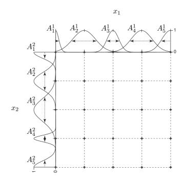
**Figure 4-4:** In the fixed fuzzy controller a grid partitioning is created through fixed membership functions. Each crosspoint corresponds with a rule consequent which defines the control output.
