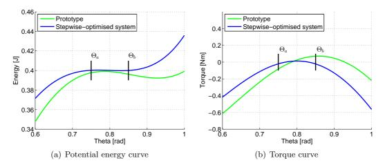
**Figure 5-7:** The potential energy and torque curves of the spring mechanism with both the prototype and the two optimised system parameter values. The goal of the optimisation was to minimise torque applied by the spring mechanism between the angles  $\Theta_a$  and  $\Theta_b$ . This corresponds with a minimisation of the derivative of the potential energy curve.
