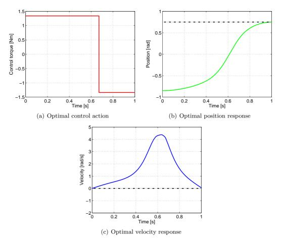
**Figure 5-8:** The optimal control solution for the 1-DOF RA with optimised system parameters when starting from an initial state of  $[\Theta, \dot{\Theta}] = [-0.85, 0]$  and moving towards the closest boundary of the place state at  $[\Theta_d, \dot{\Theta}_d] = [0.75, 0.05]$ .
