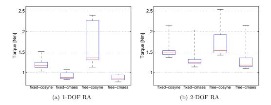
**Figure 5-16:** Boxplots representing the lower quartile, median, upper quartile, the smallest and largest sample of the minimised torques of 20 solutions found for each of the four different controller-algorithm combinations.
