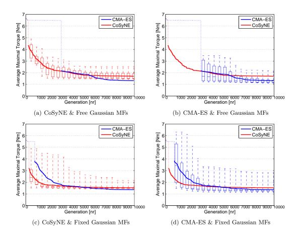
**Figure 5-18:** The convergence of the four controller-algorithm combinations for the 2-DOF RA experiment. The plotted line represents the median of 20 runs and the box represents the lower quartile and the upper quartile, the lines connected to the box show the smallest and largest sample. Although CoSyNE shows a quicker convergence for the free fuzzy controller, the CMA-ES algorithm is able to converge to a better solution for both types of controllers.
