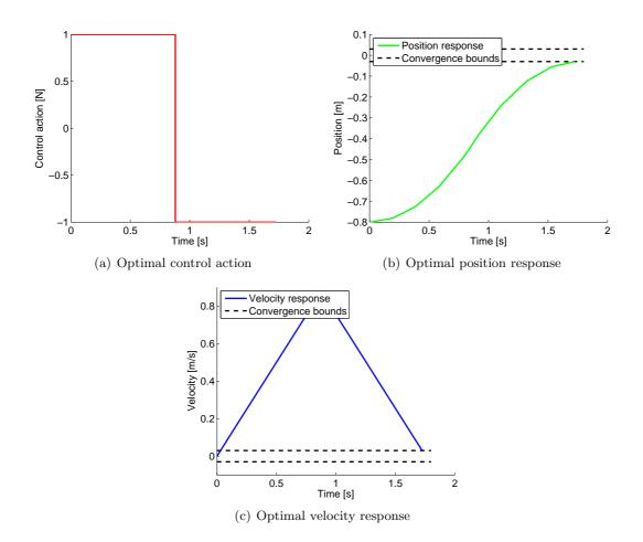
**Figure 5-4:** The optimal control output and state response for a minimal time frictionless mass control problem when starting from  $[z, \dot{z}] = [-0.8, 0]$ . The bang-bang controller generates a switching behaviour from +1 to -1 at half of the convergence time.
