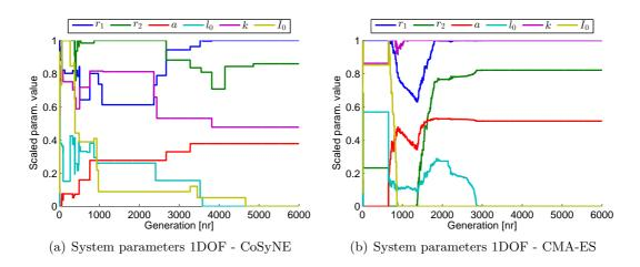
**Figure 5-19:** The normalised system parameters plotted for each generation when optimised by the CoSyNE and CMA-ES algorithm. In these plots 0 represents the lower bound and 1 the upper bound of the particular system parameter. The figures show that the CMA-ES algorithm is able to give a faster convergence to a system parameter solution while the CoSyNE algorithm is changing the system parameters with bigger steps and does not converge as quickly.
