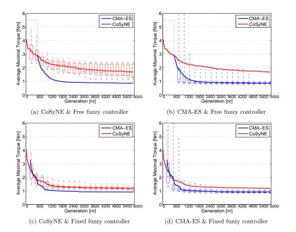
**Figure 5-17:** The convergence of the four controller-algorithm combinations for the 1-DOF RA experiment. The plotted line represents the median of 20 runs and the box represents the lower quartile and the upper quartile, the lines connected to the box show the smallest and largest sample. Although CoSyNE shows a faster initial convergence for the free fuzzy controller, the CMA-ES algorithm is able to converge to a better solution for both types of controllers.
