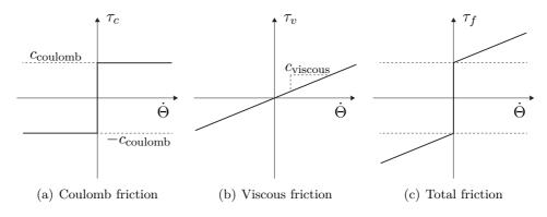
**Figure 3-5:** The friction in the Resonating Arm is modelled as a static coulomb friction (a) with friction coefficient  $c_{\text{coulomb}}$  and a dynamic viscous friction (b) with friction coefficient  $c_{\text{viscous}}$ . The coulomb friction is a constant friction independent of the velocity  $\dot{\Theta}$ , while the viscous friction is depending on the velocity  $\dot{\Theta}$ . The total friction (c) is the sum of both friction types.
