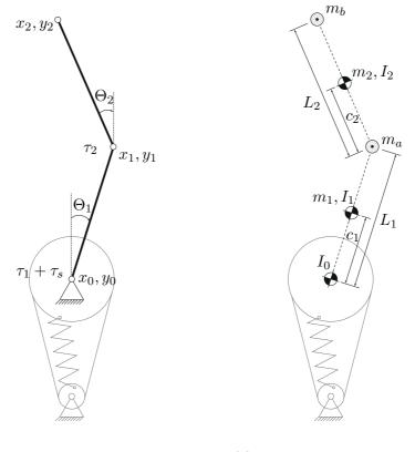
(a) State variables and torques (b) Center of masses and inertia
