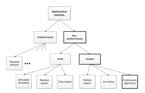
**Figure 2-1:** A classification of optimisation methods in gradient-based, non-gradient-base, serial and parallel methods with examples of common methods.
