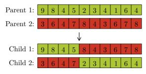
Figure 2-3: Single-point crossover operator.
