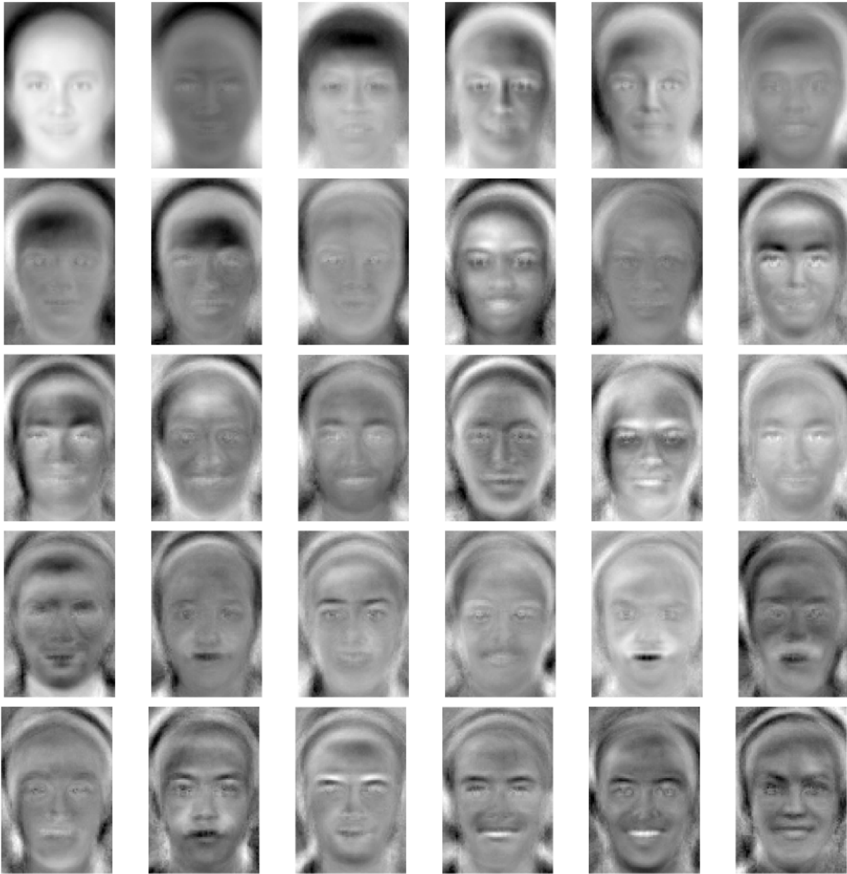
Fig. 5. The first 30 eigenfaces derived by the Eigenfaces method. The order of these vectors is listed from left to right and top to bottom corresponding to the eigenvalues in decreasing order.
