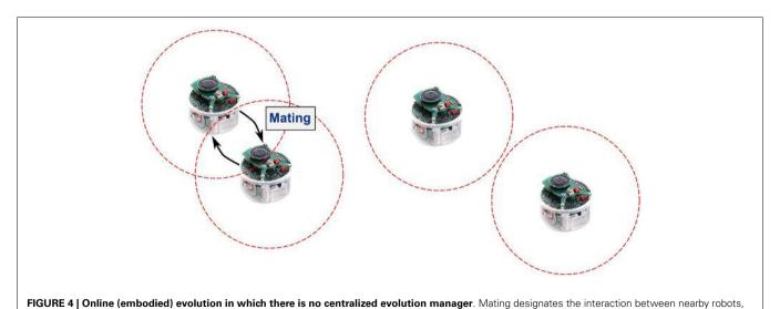
when genotypic information is exchanged. Evaluation, selection, and variation operations are then performed onboard each single robot, in a distributed manner.
