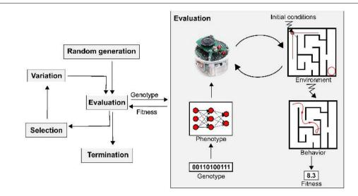
FIGURE 1 | Principal workflow of evolutionary robotics. The diagram presents a classic evolutionary robotics system, which consists of an evolutionary algorithm (left) and a robot, real or simulated (right). The evolutionary component follows the generic evolutionary algorithm template with one application-specific feature: for fitness evaluations, the (real or simulated) robot is invoked. The
