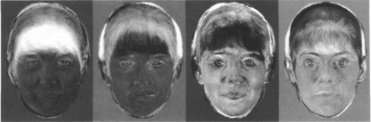
Figure 1. The first four eigenfaces from this set of 20 faces. These are deviations from the average face, with zero coded as a mid gray level and black and white as opposite extremes.
