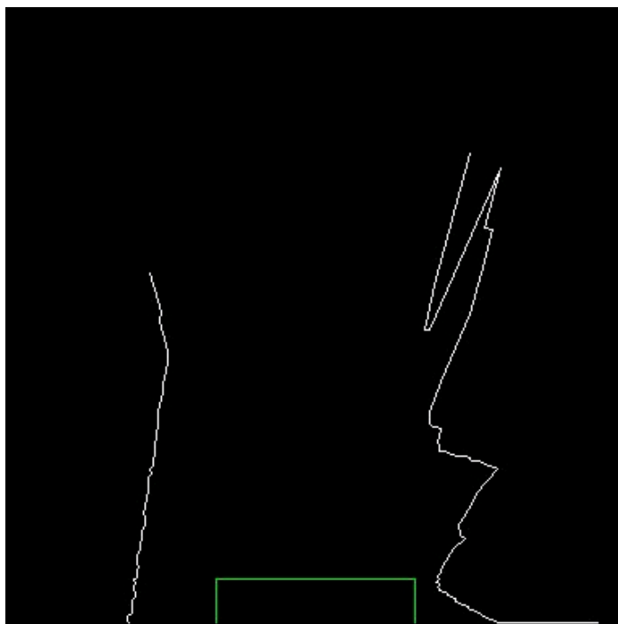
Figure 4. “Zoom mode” showing the front of the robot (the rectangle in the bottom of the figure) and lines indicating obstacles in the area immediately around the robot.
