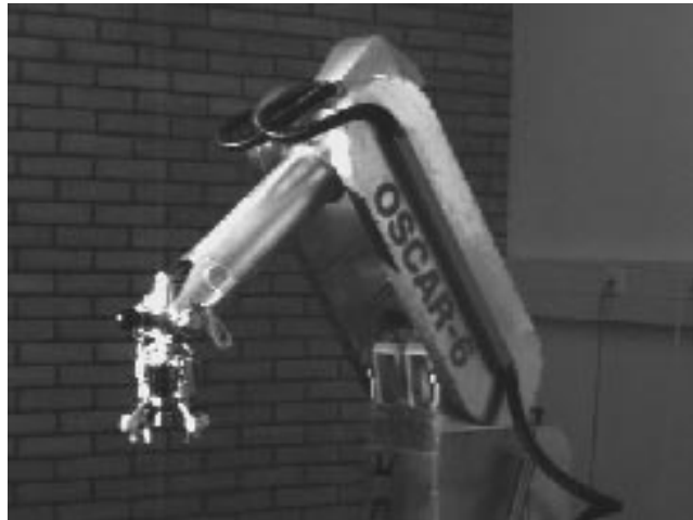
Figure 1: The OSCAR-6 robot arm. OSCAR is designed for pick-and-place tasks and has been applied in several industrial settings. The arm contains 6 total joints and a camera mounted in the end effector.
