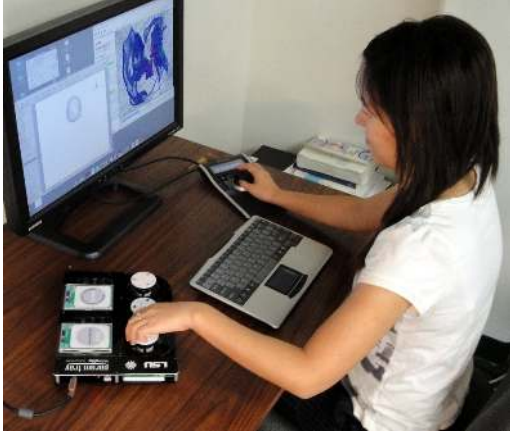
Figure 6: User physically manipulating VISH application through “viz tangibles” interaction devices
