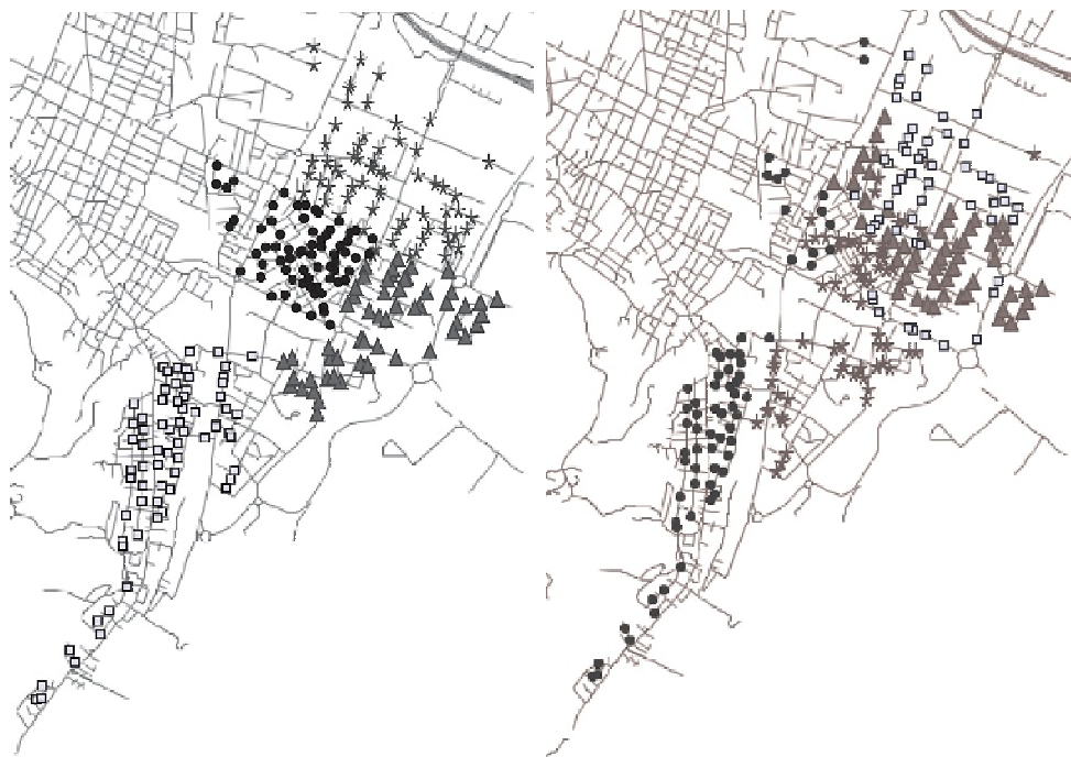
Figure 6 Comparison between hand-made and heuristic solutions of a real-world waste collection problem with four routes. The hand-made solution (left) is about 4% longer but more compact than the heuristic one (right).
