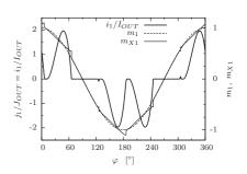
Mode 4, waveforms of  $i_1$ ,  $v_1$ , and  $v_{X1}$ ,  $M_{OUT} = 1$
