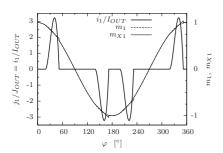
Mode 3, waveforms of  $i_1$ ,  $v_1$ , and  $v_{X1}$ ,  $M_{OUT} = 1.5$
