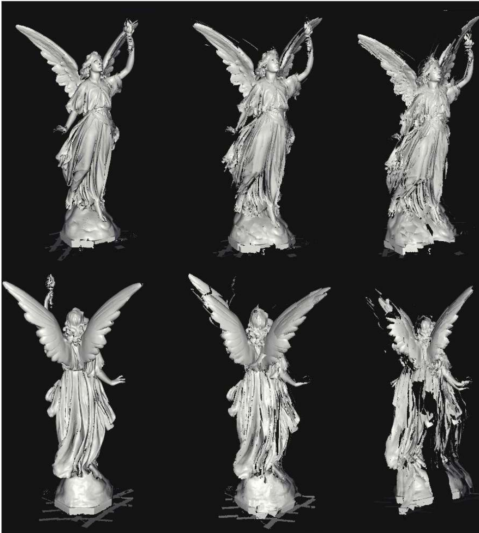
FIG. 9: Front and back views of the reconstructions from the Lucy dataset. The left one is the best found reconstruction. The middle and right ones are obtained by LUD and EIG.
