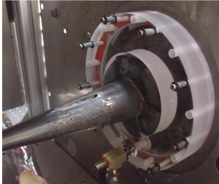
Figure 65: Installed quartz back plate
