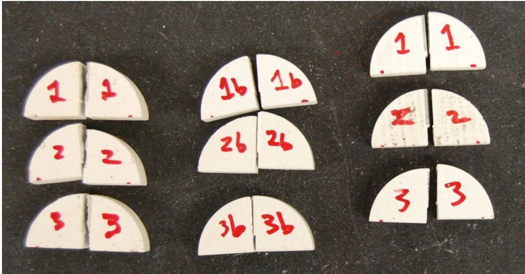
Figure 11. Gypsum plaster SCB specimens after testing. The samples on the left contain Berea sandstone discontinuities. The samples in the middle contain gypsum plaster discontinuities. And, the samples on the right contain glass discontinuities.
