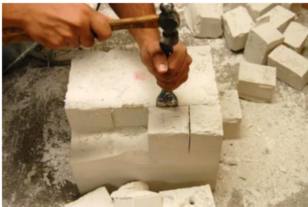
Figure 8. The dismantling of a specimen by chiseling after hydraulic fracturing.
