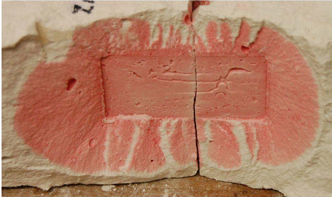
Figure 31. Test 3a exhibiting a roughly orthogonal intersection between a hydraulic fracture (propagating out of the page) and a plaster slide (seen by the rectangular outline). There is mode I-II propagation to the right and left of the natural fracture, and there is mode I-III propagation above and below the natural fracture. As seen, the mode I-III en echelon cracks propagate in directions that are mirror images of each other across the hydraulic fracture / natural fracture line of intersection.
