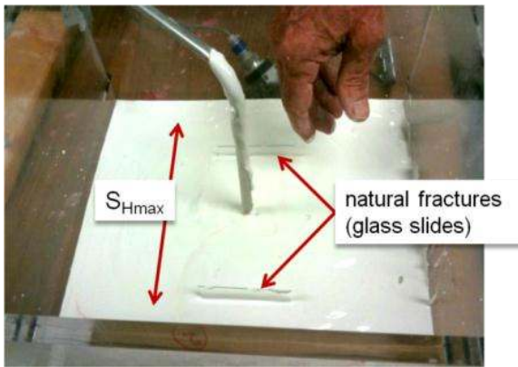
Figure 4. A test block in preparation with two glass slides set in the middle layer of plaster as it is being poured.
