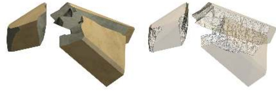
Figure 12: Advantages of the volumetric mesh. The simulation algorithm generates true 3D crack surfaces for realistic rendering. Left: A tile being broken in generates four detailed surface meshes. Right: Visualization of these meshes.
