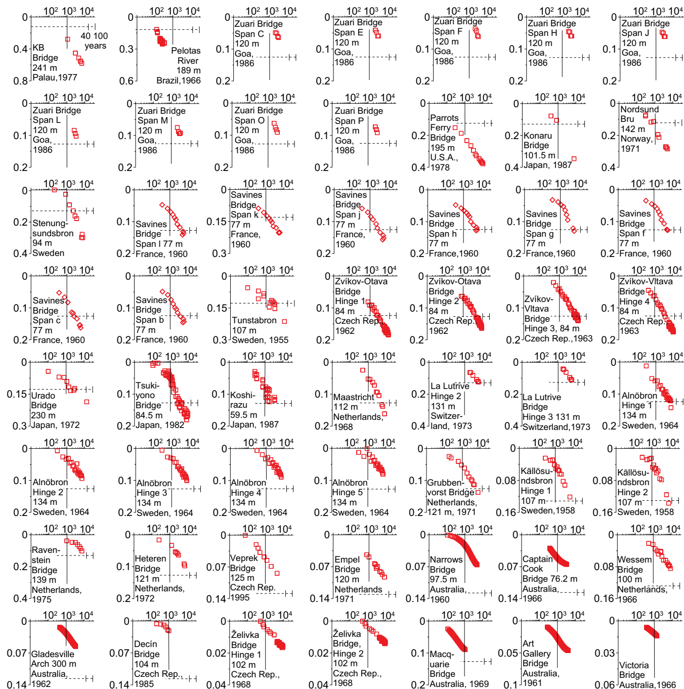
Fig. 1: Excessive deflections measured on 56 segmental bridge spans. Ordinates are deflection-span ratios, %; abscissas are time, days. Each horizontal dashed line corresponds to a deflection of 1/800 of the span, considered the maximum allowable. The associated vertical tick marks respectively indicate times of 40 and 100 years after span closing. Data were obtained from private communications with Yasumitsu Watanabe, Shimizu Corp., Tokyo; Jan Vitek, Metrostav, Prague; Vladimír Křístek and Lukáš Vráblík, CTU Prague; and Miloš Zich, Brno; as well as from References 6 through 12
