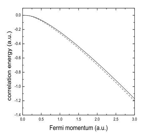
FIG. 4: Correlation energy for Ps in an electron gas as a function of the Fermi momentum  $k_F$ . Solid line, Ps momentum p = 0.2 a.u. Dashed line, p = 1.0 a.u.
