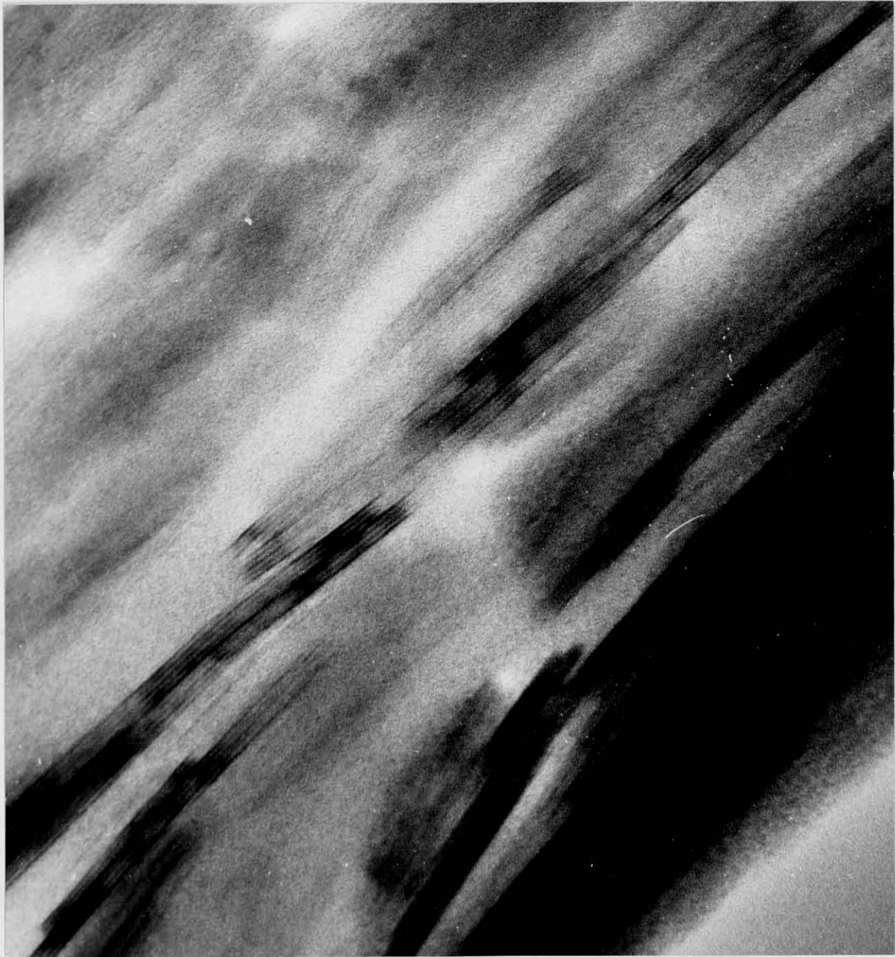
Fig. 1. High resolution electron micrograph of \text{Cs}^+ saturated micaceous vermiculite from Marblehead, Wisconsin: The micrograph shows 10.3\text{\AA} spacings which represent structural images of the (001) cleavage surfaces of the micaceous phase. The presence of occasional darker fringes in a particle indicate that the adsorbed \text{Cs}^+ in interlayer exchange sites have enhanced the contrast of the image through the higher nuclear density of \text{Cs}^+ than \text{K}^+ (Magnification of micrograph is 996,000X). From Jackson et al. (1974).
