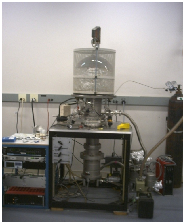
Figure 2.2 Thermal evaporation system used for making all thin films reported in this thesis.
