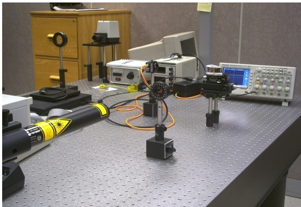
Figure 3.2 Kretschmann configuration set-ups on an optical table.
