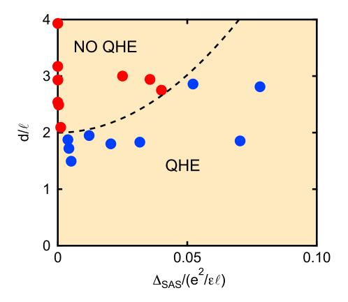
FIG. 3: Phase diagram of the  $\nu_T=1$  bilayer 2DES system in the  $d/\ell - \Delta_{SAS}/(e^2/\epsilon\ell)$  plane. Blue circles: Bilayer samples which display a quantized Hall plateau at  $\rho_{xy}=h/e^2$  at  $\nu_T=1$ . Red circles: Samples which do not display a quantized Hall plateau at  $\nu_T=1$ . This figure strongly suggests that the  $\nu_T=1$  QHE persists even in the limit of zero tunneling. After Murphy et al. [21].
