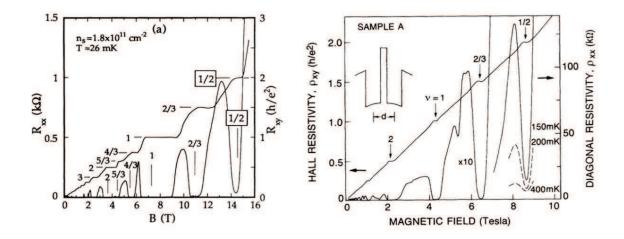
FIG. 1: Discovery of quantized Hall states at  $\nu_T = 1$  and  $\nu_T = 1/2$  in bilayer electron systems. In the left panel the bilayer system is realized in a wide single quantum well, while on the right the electrons reside in a double quantum well. After Suen *et al.* [1] and Eisenstein *et al.* [2].
