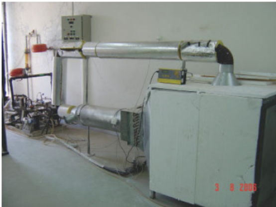
Figure 2: Outside view of the GSHP drying system investigated
