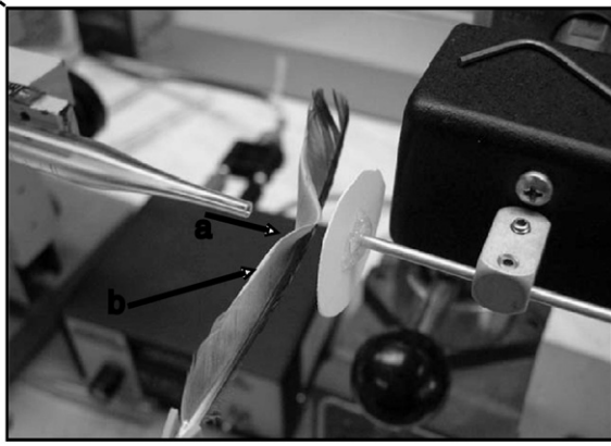
Fig. 2. Set up for the barbicular hooking strength test; (a) direction of pressurized air; (b) feather vane.
