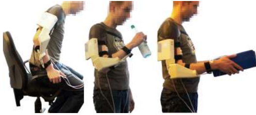
FIGURE 2: The patient is able to train independently various types of exercise of daily life. A special shoulder strap increases the stable seating of the orthosis, resulting in a better weight distribution.
