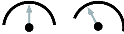
Fig. 3. We manipulate the mapping between head rotation and virtual display position, here seen from above the user, with the arrow indicating the user head rotation and the arc being the virtual displays. Left : The user looks straight ahead at the central display of a workspace. Right : As the user's head rotates to the left, the virtual displays rotate to the right; i.e., they counter-rotate, with the extent of this counter-rotation determined by the mapping in use.
