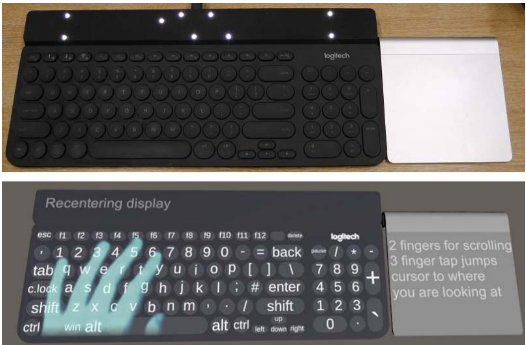
Fig. 15. Closeup of (top) the physical Logitech Mixed Reality keyboard and attached Apple Magic Trackpad and (bottom) virtual equivalents in VR with hand visualization on the keyboard.
