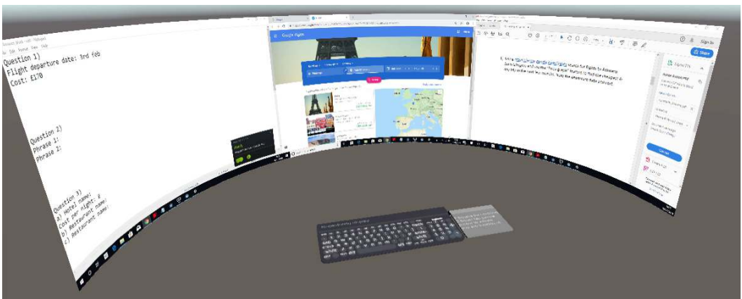
Fig. 14. Three display virtual workspace with positionally tracked keyboard and trackpad, with the holiday planning task applications open and assigned to each display (from left: notepad, browser, pdf viewer).
